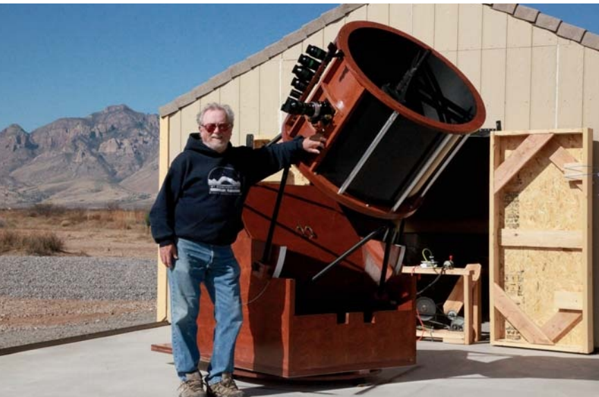
Phill Oltmann with his 32-inch f/2.4 scope. The scope stays put while the observatory rolls away from it, using the same motor that powered the polishing process.
